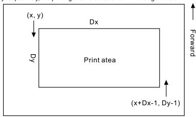
• This printable area for this printer is approximately 72 mm in the horizontal direction and approximately 117.3 mm (1662/360 inches) in the vertical direction.
