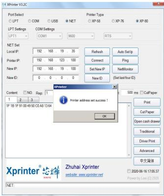
4. After the prompt window indicating "printer address successfully set" appears, print self test page again to see if the IP address has been modified, as shown in the picture below:
